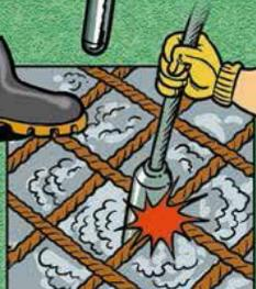
EVITAR O CONTACTO DO VIBRADOR COM AS ARMADURAS E/OU A COFRAGEM.
